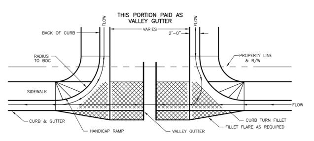
NOTE: PROVIDE 1-FOOT FLARE WHEN FILLETS ARE INSTALLED AT THE LOCATION OF VALLEY GUTTER
